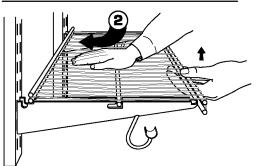
Push down and maintain pressure on center of shelf. Then lift front edge and slide shelf back ②. Shelf will snap into place.
