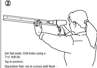
then give power drill a good burst or two (or 4 to 6 complete rotations) to pull up anchor.
